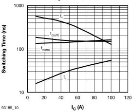
Fig. 10 - Typical IGBT Switching Time vs.  $I_C$   $T_J$  = 125 °C, L = 500  $\mu$ H,  $V_{CC}$  = 360 V,  $R_q$  = 5  $\Omega$ ,  $V_{GE}$  = 15 V
