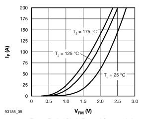
Fig. 5 - Typical Diode Forward Characteristics
