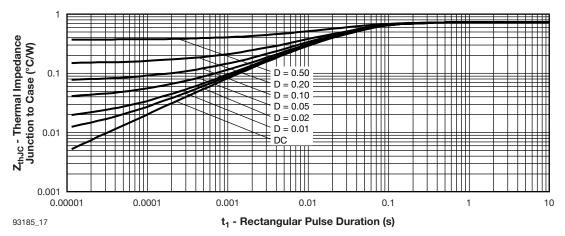
Fig. 17 - Maximum Thermal Impedance Z<sub>thJC</sub> Characteristics (Diode)
