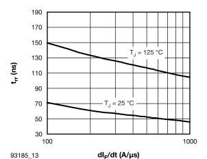
Fig. 13 - Typical  $t_{rr}$  Diode vs.  $dI_F/dt$   $V_{rr}$  = 200 V,  $I_F$  = 50 A
