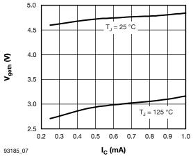
Fig. 7 - Typical IGBT Threshold Voltage
