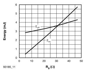
Fig. 11 - Typical IGBT Energy Loss vs.  $R_g$   $T_J$  = 125 °C,  $I_C$  = 100 A, L = 500  $\mu$ H,  $V_{CC}$  = 360 V,  $V_{GE}$  = 15 V
