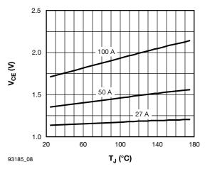
Fig. 8 - Typical IGBT Collector to Emitter Voltage vs. Junction Temperature,  $V_{\text{GE}} = 15 \text{ V}$
