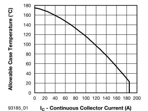
Fig. 1 - Maximum DC IGBT Collector Current vs.
