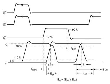
Fig. 19b - Switching Loss Waveforms Test Circuit
