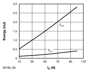
Fig. 9 - Typical IGBT Energy Loss vs. I<sub>C</sub>  $T_J$  = 125 °C, L = 500  $\mu$ H, V<sub>CC</sub> = 360 V,  $R_g$  = 5  $\Omega$ , V<sub>GE</sub> = 15 V
