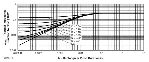
Fig. 16 - Maximum Thermal Impedance  $Z_{\text{thJC}}$  Characteristics (IGBT)
