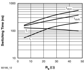
Fig. 12 - Typical IGBT Switching Time vs.  $R_g$   $T_J$  = 125 °C, L = 500  $\mu$ H,  $V_{CC}$  = 360 V,  $I_C$  = 100 A,  $V_{GE}$  = 15 V
