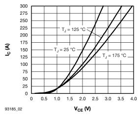
Fig. 3 - Typical IGBT Collector Current Characteristics  $V_{\text{GE}} = 15 \text{ V}$
