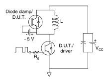
Fig. 19a - Switching Loss Test Circuit
