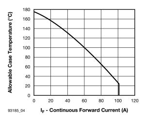
Fig. 4 - Maximum DC Forward Current vs. Case Temperature
