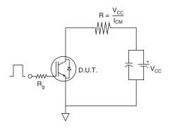
Fig. 18b - Pulsed Collector Current Test Circuit
